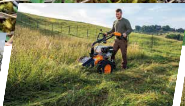
Gentle cut with double knife cutter bar
