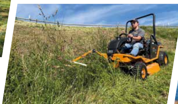
Insect-friendly Mowing with insect scare device
