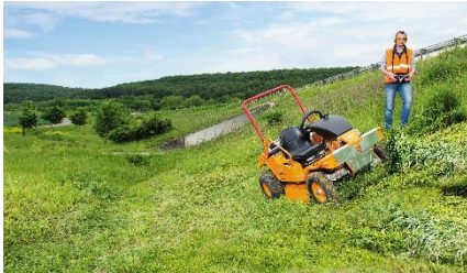
Photo 5: AS 940 Sherpa 4WD RC in use on a slope along a guard rail.
